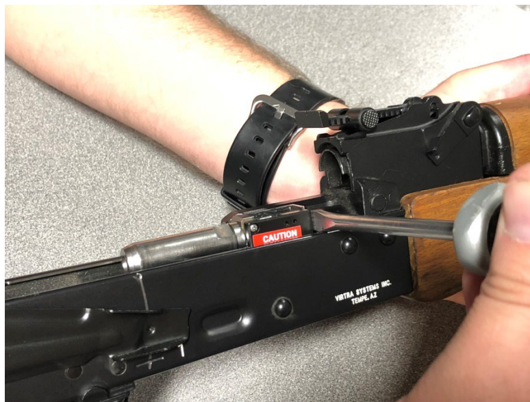
Figure 12: DO NOT PRY AT THIS LOCATION
