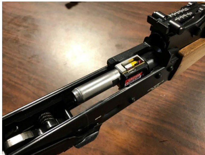
Figure 2: Charge Chamber Installation
