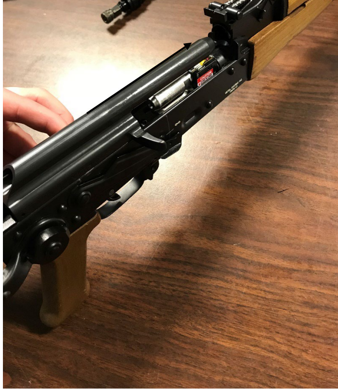
Figure 5: Bolt Carrier Installation 1
