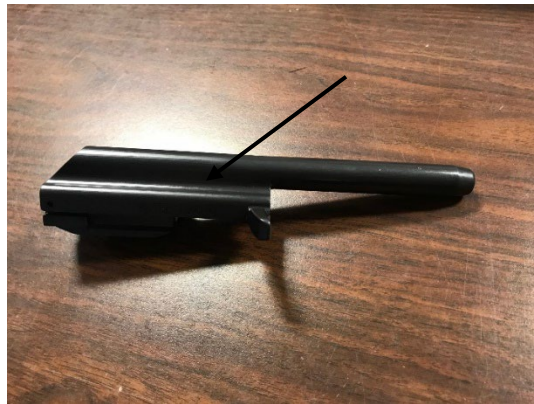
Figure 4: Bolt Carrier Lubrication
