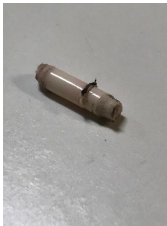
Figure 4: Damaged Air Tube
