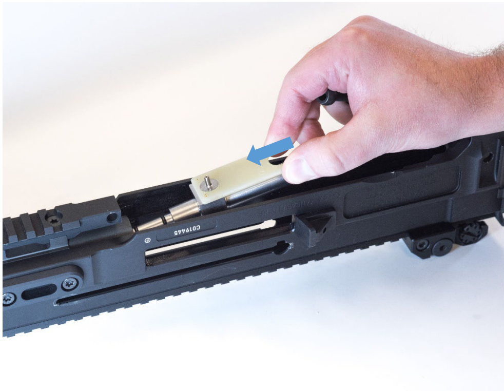
Figure 9: Charge Chamber Install
