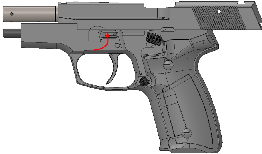
Figure 7: Installation of Slide onto Frame (3 of 3)
