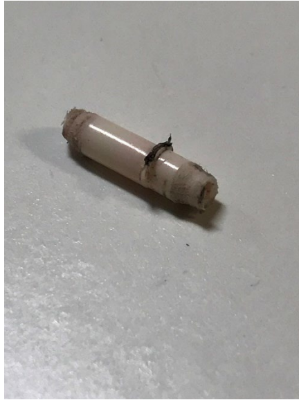
Figure 8: Damaged Air Tube
