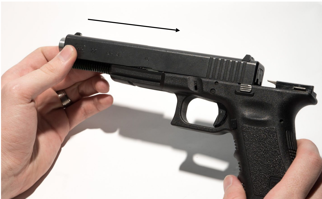
Figure 6: Handgun Frame Install
