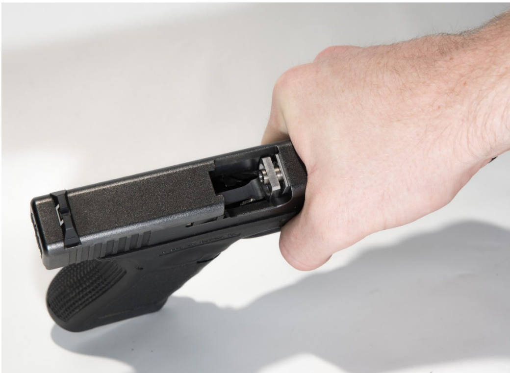
Figure 8: Completed Tailpiece Install
