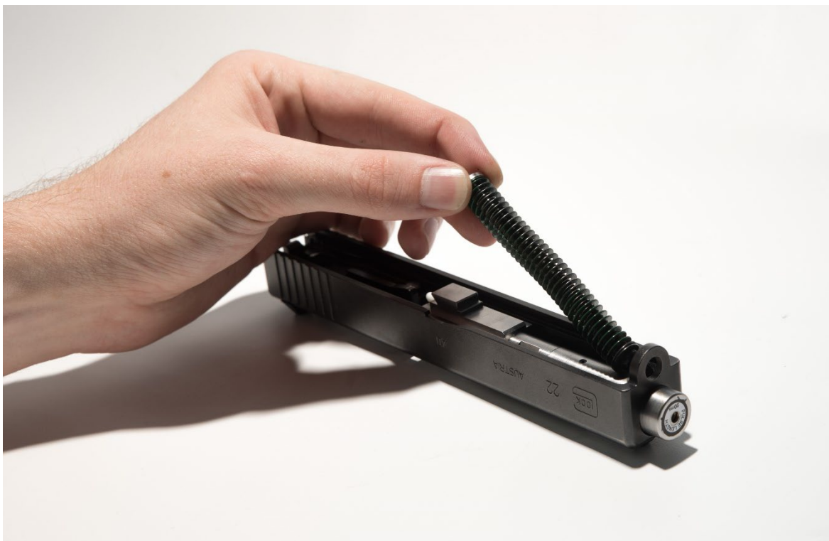
Figure 4: Recoil Spring Install
