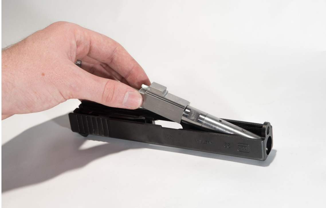
Figure 3: Barrel Assembly Install
