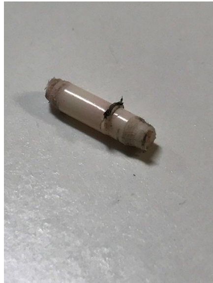
Figure 7: Damaged Air Tube
