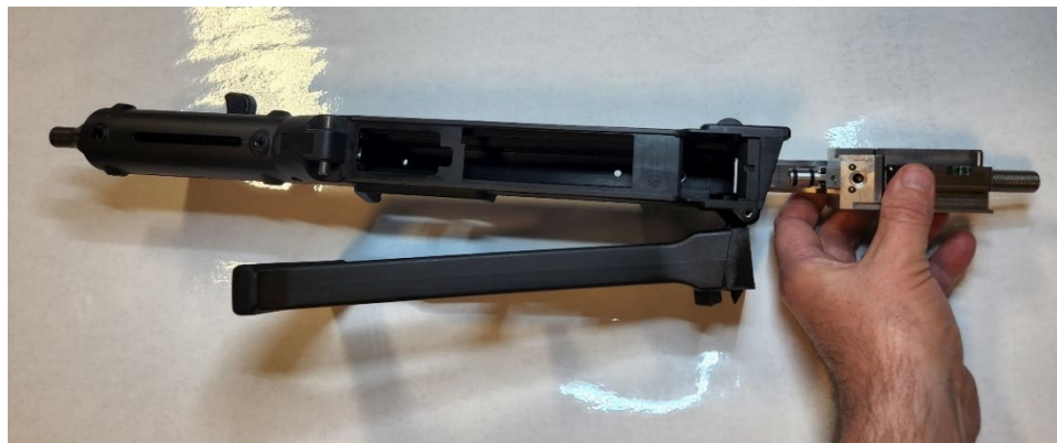
Figure 10, Orientation of Recoil-Kit into firearm.
