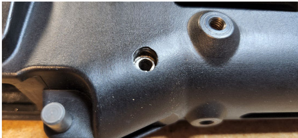
Figure 8, UMP Barrel Roll Pin properly installed.
