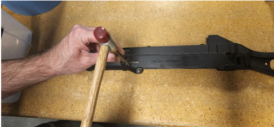
Figure 2, Remove UMP Barrel Roll Pin.
