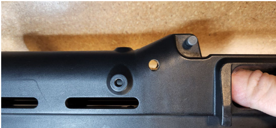
Figure 6, Align hole in receiver with slot in barrel.
