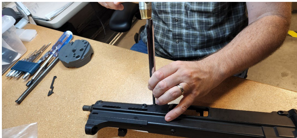
Figure 7, Re-insert UMP Barrel Roll Pin.
