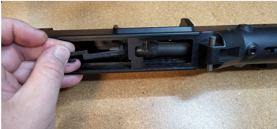
Figure 4, Remove ejector lever.
