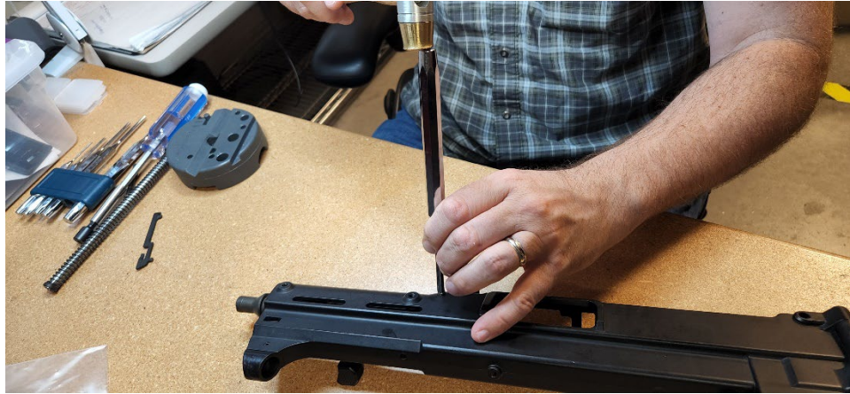
Figure 7, Re-insert UMP Barrel Roll Pin.
