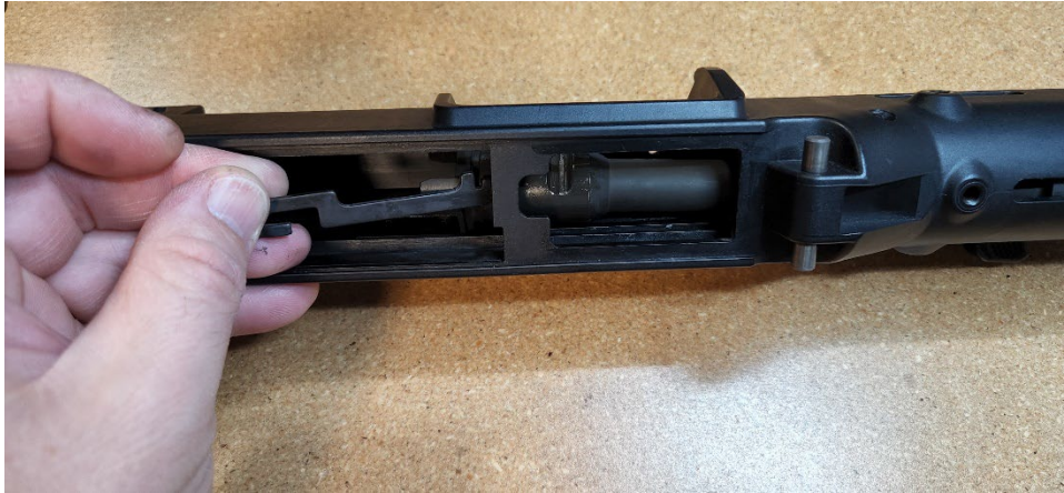
Figure 4, Remove ejector lever.
