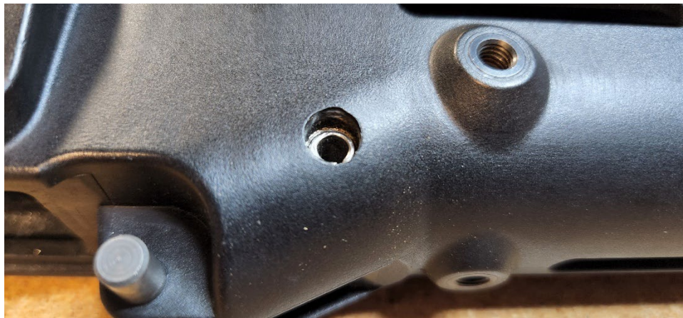
Figure 8, UMP Barrel Roll Pin properly installed.
