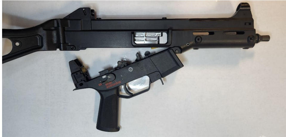
Figure 14, Re-attach Lower Receiver taking care not to bend gold pogo-pins.
