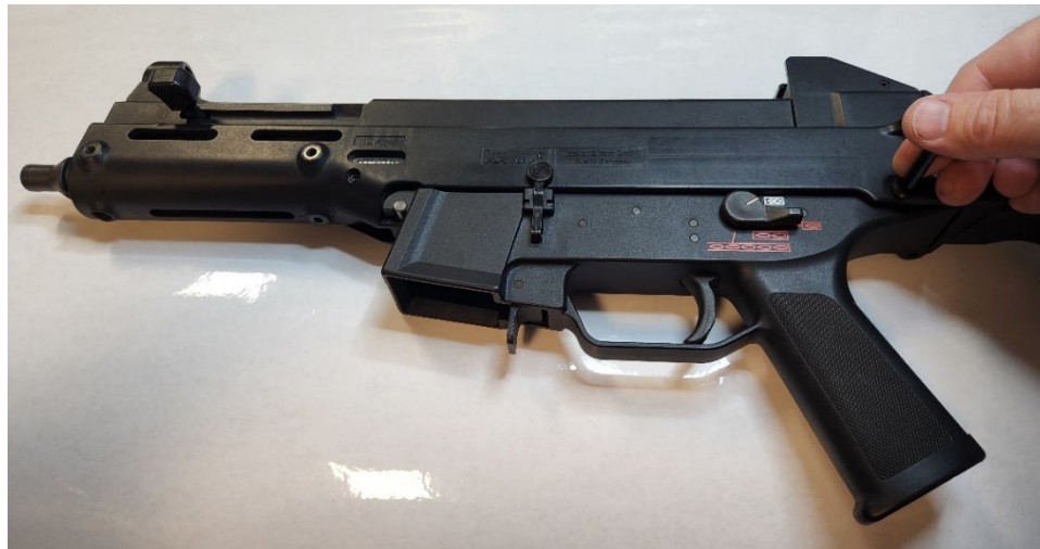
Figure 15, Insert Take-Down pin.
