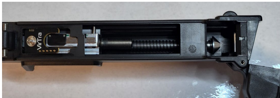
Figure 13, Insert the Recoil Spring.
