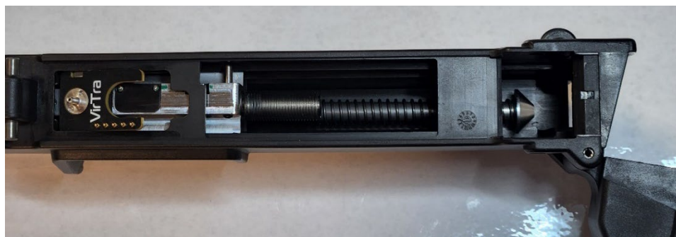
Figure 13, Insert the Recoil Spring.
