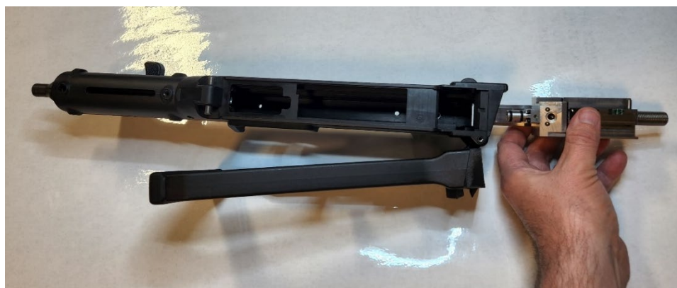
Figure 10, Orientation of Recoil-Kit into firearm.
