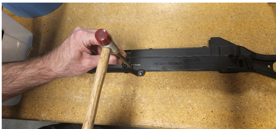
Figure 2, Remove UMP Barrel Roll Pin.
