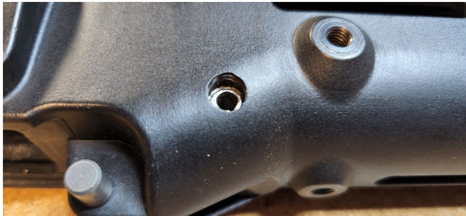
Figure 8, UMP Barrel Roll Pin properly installed.
