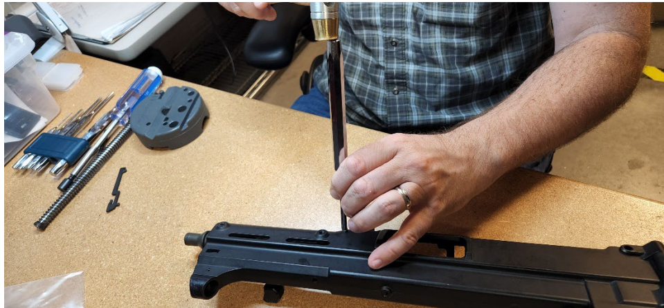
Figure 7, Re-insert UMP Barrel Roll Pin.
