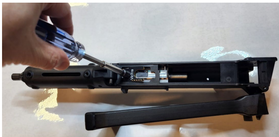
Figure 12, Install Retaining Plate by threading in Charge Chamber Nipple.
