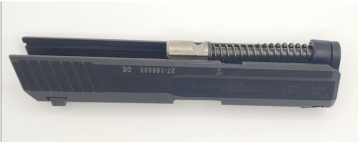
Figure 5: Completed Recoil Spring Install
