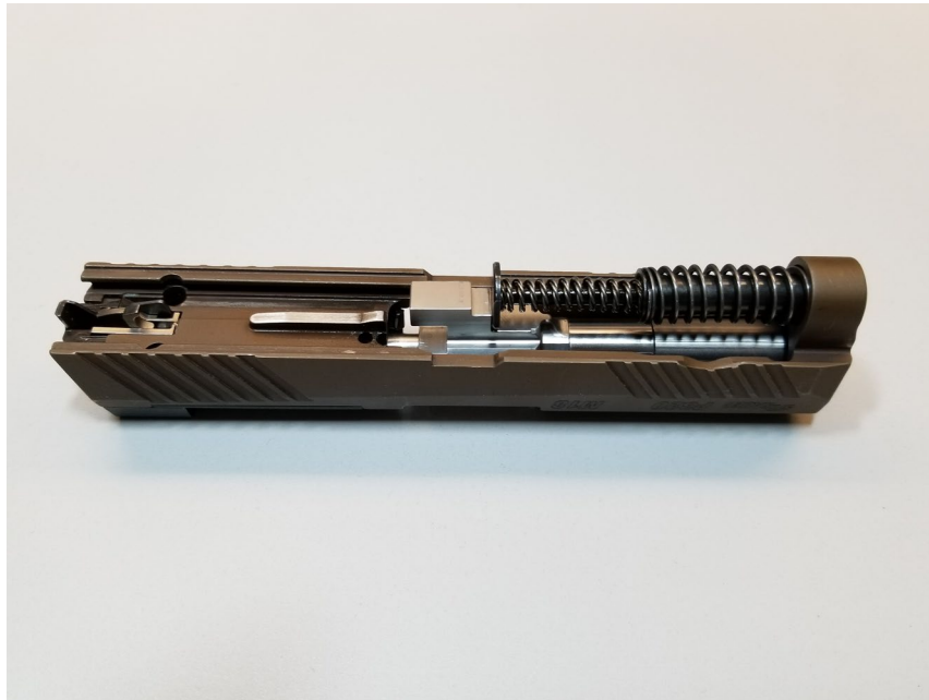
Figure 5: Completed Recoil Spring Install
