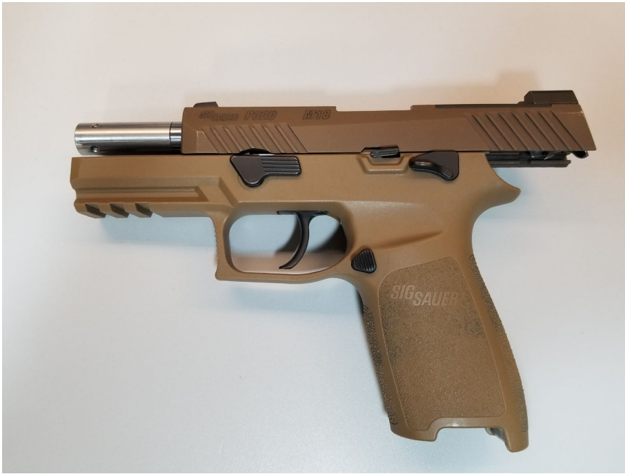
Figure 7: Slide Lock Rotated
