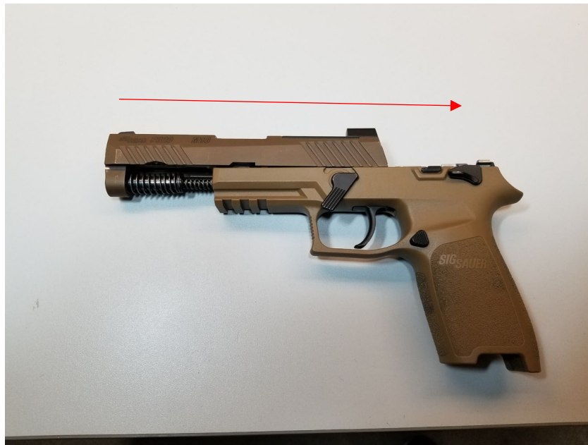
Figure 6: Handgun Frame Install
