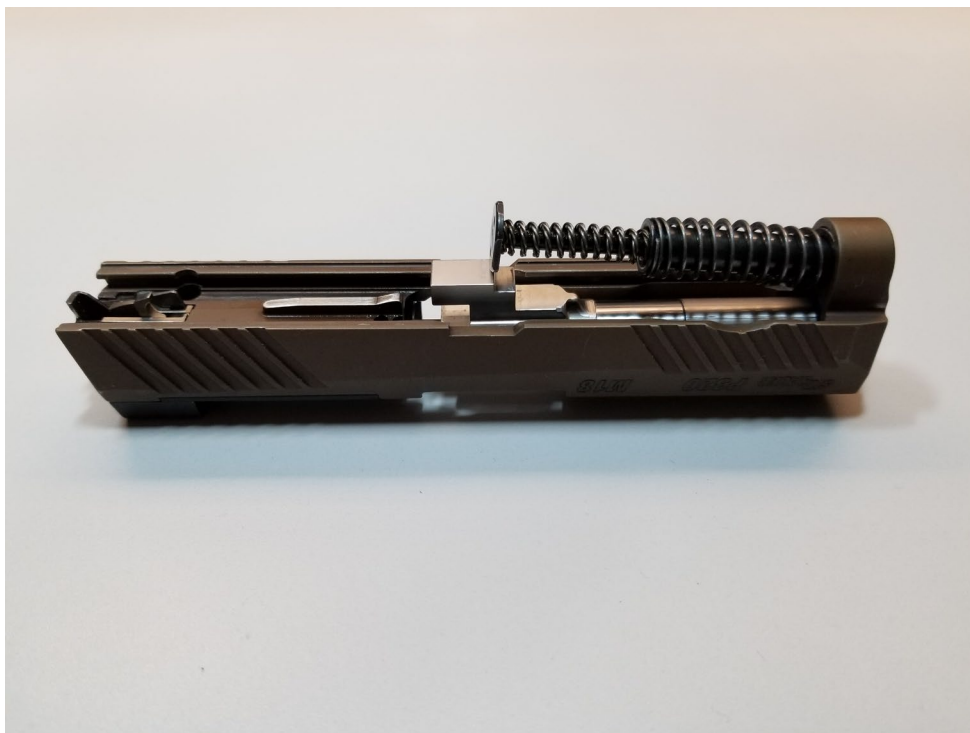
Figure 4: Recoil Spring Install
