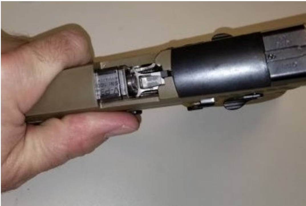
Figure 9: Completed Tailpiece Install
