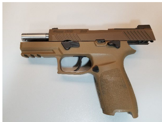
Figure 6: slide in lock position
