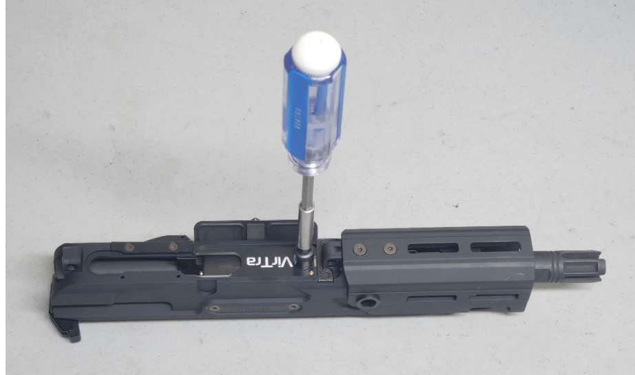
Figure 5, Install the retaining plate and screw in the Charge Chamber Nipple.
