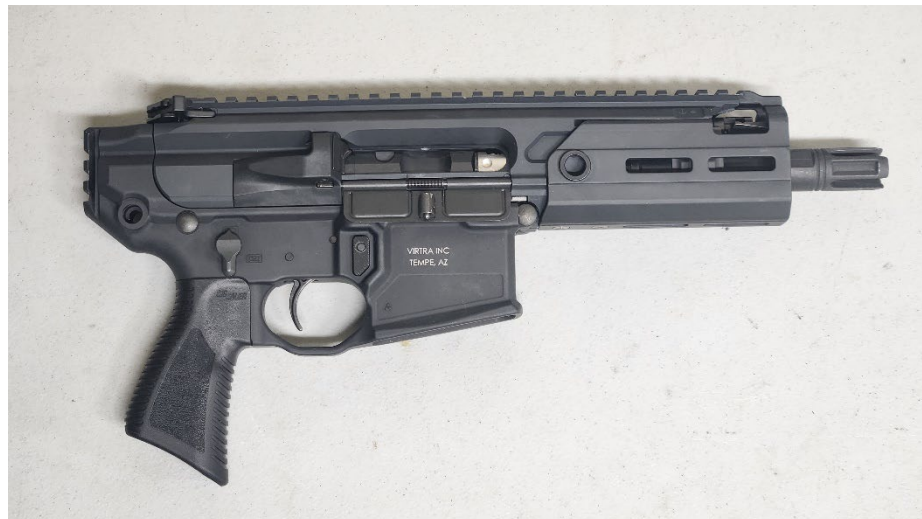
Figure 6, Re-attach the upper and lower receivers.
