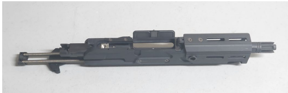
Figure 4, Recoil Kit inserted into MCX Upper Receiver.
