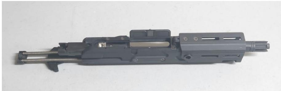
Figure 4, Recoil Kit inserted into MCX Upper Receiver.
