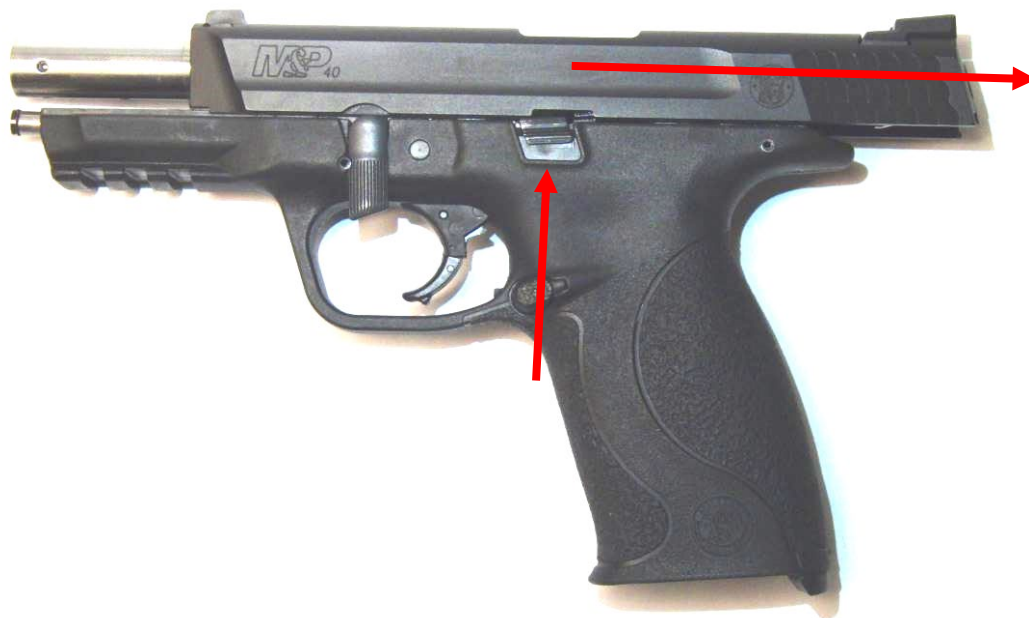
Figure 6: Installation of Slide onto Frame (2 of 3)
