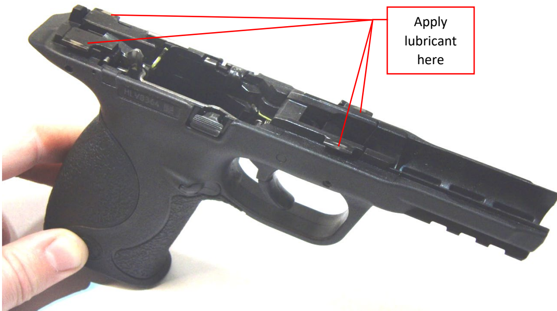
Figure 3: Lubrication of Frame Rails
