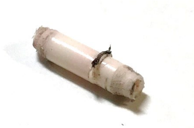
Figure 7: Damaged Air Tube
