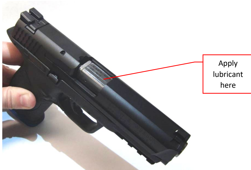
Figure 4: Lubrication of Recoil Kit thru Ejection Port
