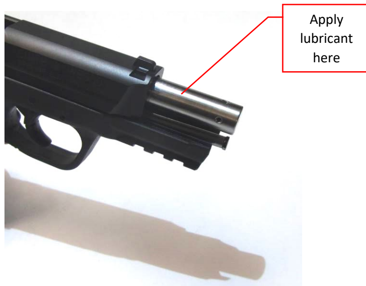
Figure 5: Lubrication of Recoil Kit Barrel
