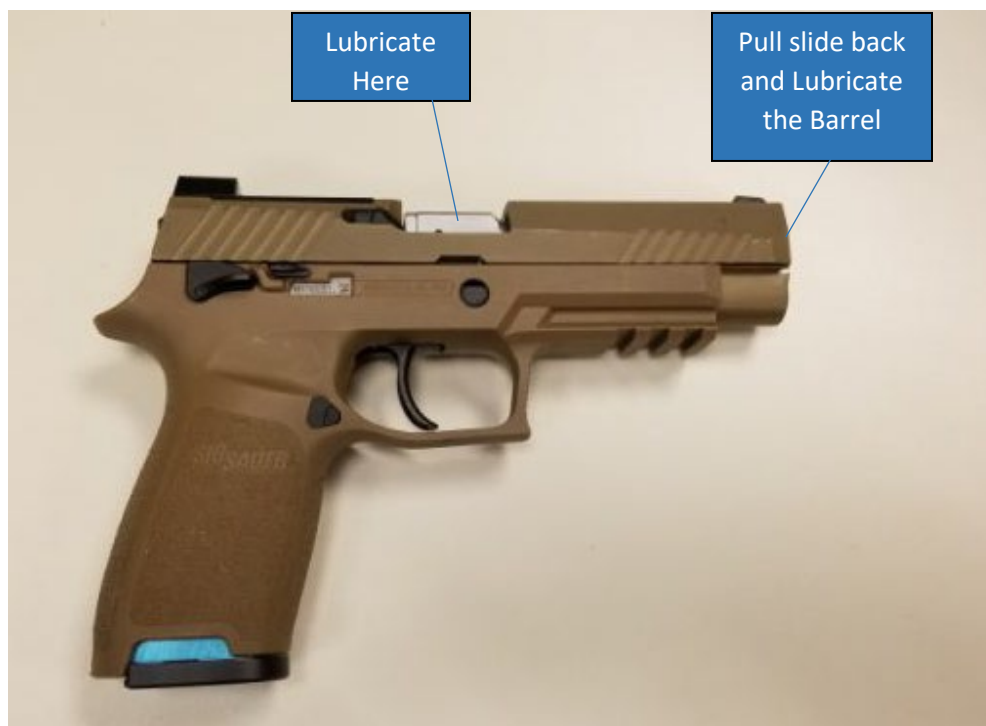
Figure 3: Ejection Port and Barrel Lubrication
