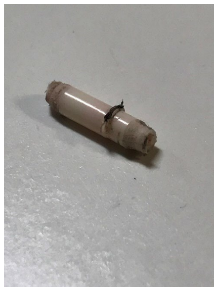
Figure 7: Damaged Air Tube
