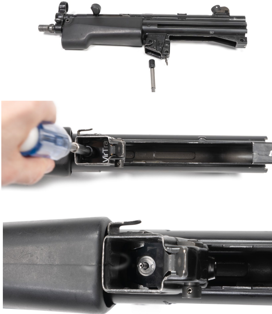
Figure 5: Charge Chamber Nipple Tightening
