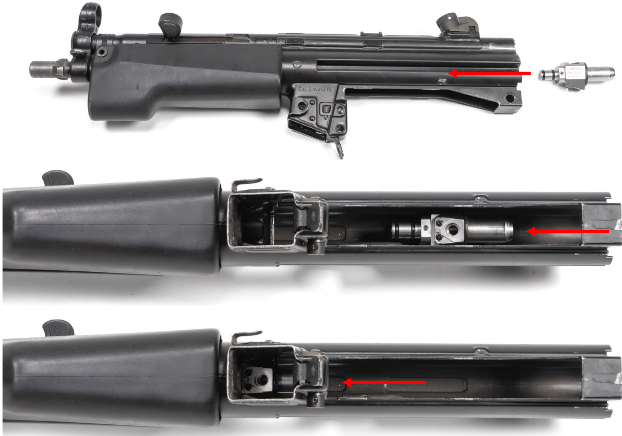
Figure 3: Charge Chamber Installation
