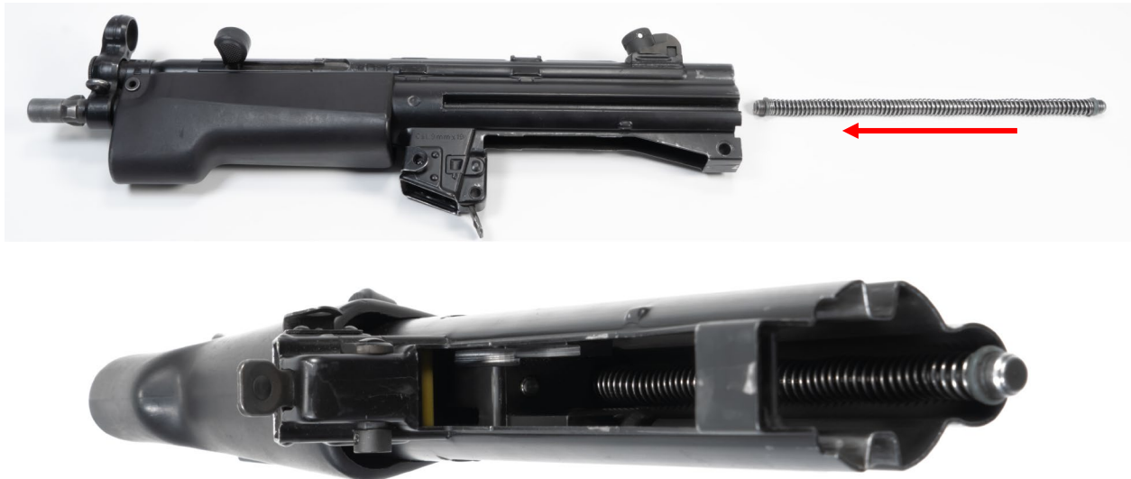
Figure 7: Factory Recoil Spring and Guide Rod Assembly Installation
