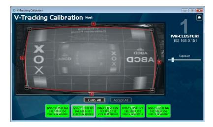
When running in host mode the calibration tool shows an alternate user interface that allows for individual control of each connected image generator system.
