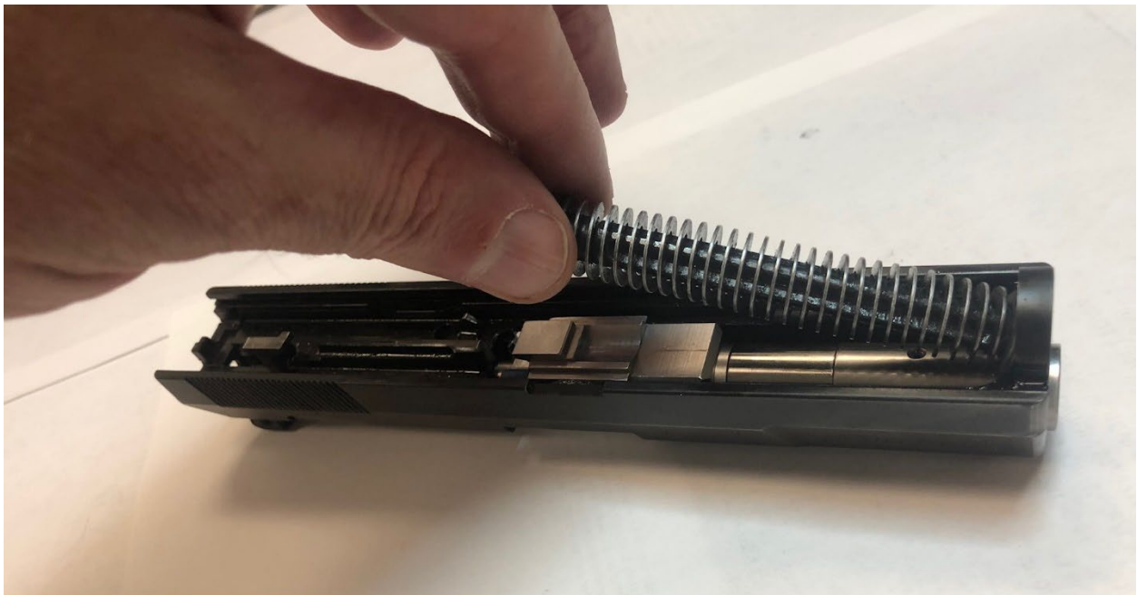
Figure 4: Recoil Spring Install
