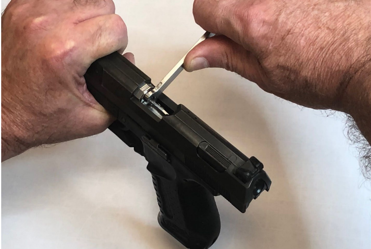
Figure 9: Tailpiece Fastener Install
