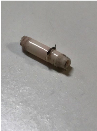
Figure 4: Damaged Air Tube
